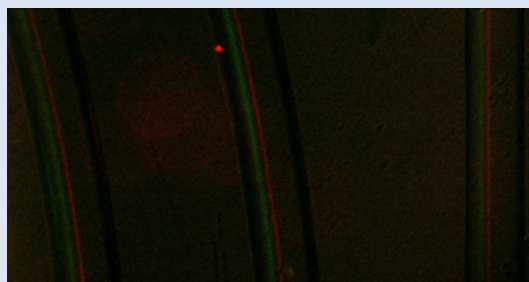
Fig. 7: Composite images illustrating the position of the 15 \mu\text{m} (green fluorescence), and 7.3 \mu\text{m} (red fluorescence) diameter particles in the channel section prior to the outlet of unit 3 of the microfluidic device. Flow rate: 150 \mu\text{l}/\text{min} .
