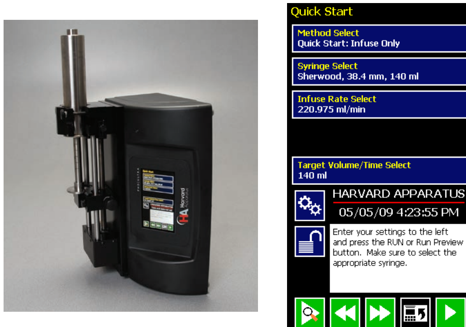
The PHD ULTRA™ 4400 pump shown in its vertical (upright) orientation and the associated Quick Start menu screen showing the application auto-rotated into portrait mode.
